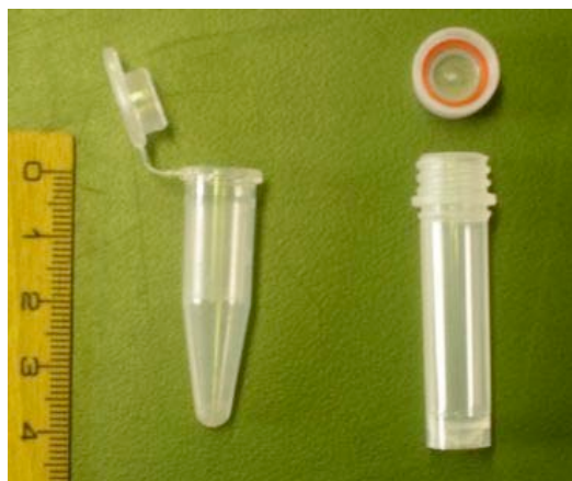
Photo 28: Typical tubes for storing samples (left: an Eppendorf tube, ref. Bioblock B51633; right: a Micrew screw tube with seal, refs Bioblock B14437 and B14457).
