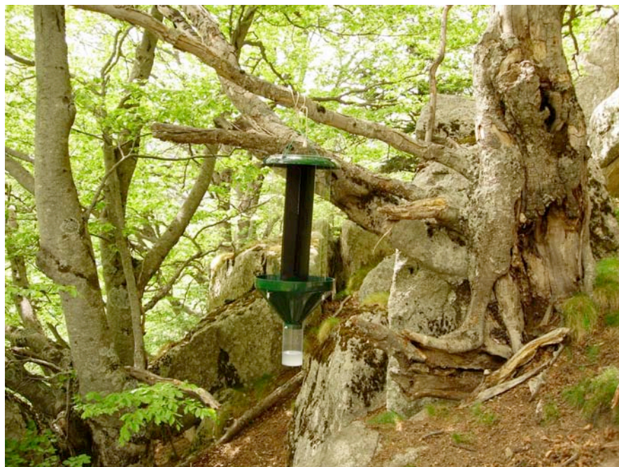
Photo 7: Black multidirectional trap (Polytrap™ type).
