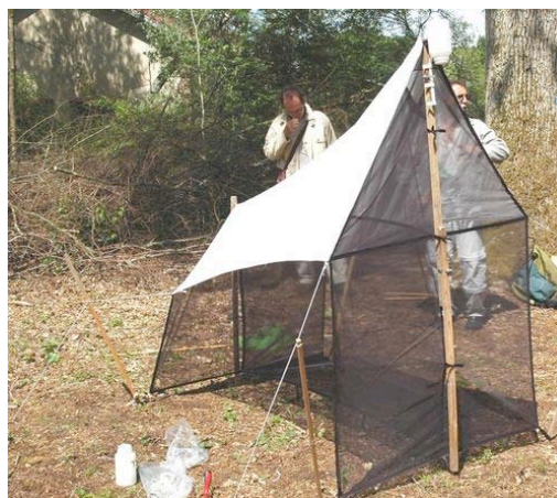
Photo 2: A typical Malaise trap
