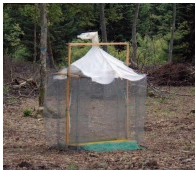
Photo 5: A composite entomological trap.
